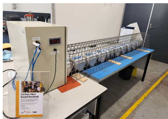
Figure 1. Custom-built Carbolt curing and heating mould with a temperature controller.
