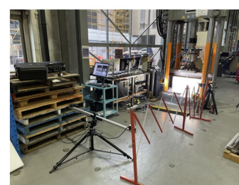
Test setup with DIC for half size sample
