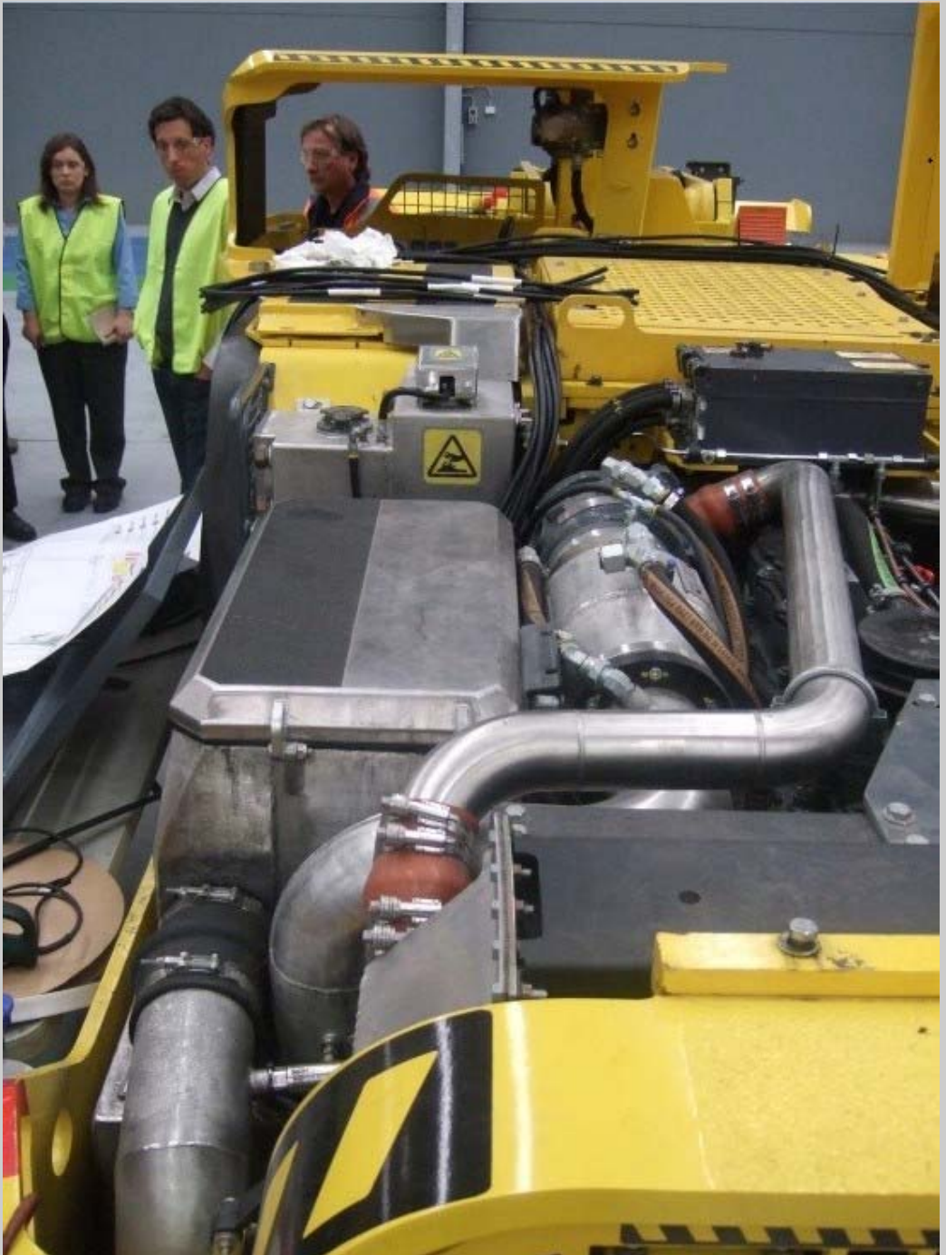
PPK COALTRAM LHD with NSW DES compliant disposable (wet element) system (and small oxidation catalyst) after treatment system
