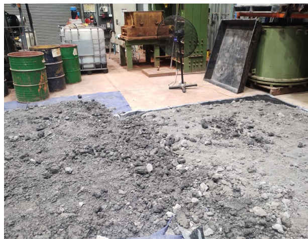
Figure 2: Material from Mine B being dried with a fan
