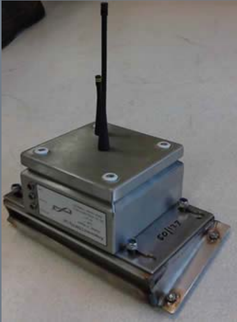
Wireless tilt monitor deployed at Austar
