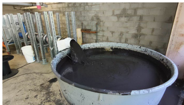
Figure 1 Dam break test using coal tailings slurry
