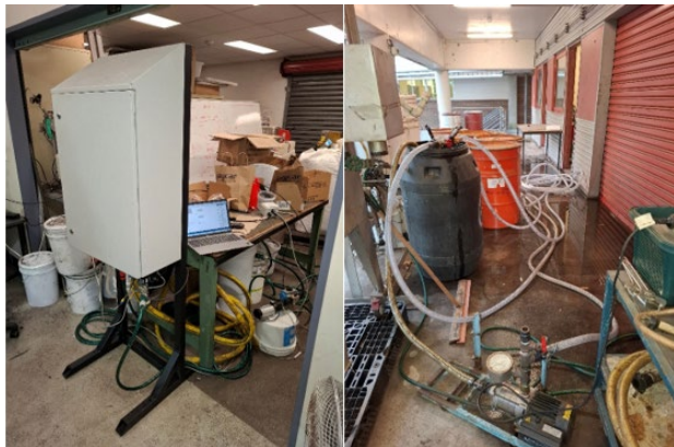
Figure 1. Particle Profiler proto-type unit mounted on frame (left) and slurry cycling equipment (right).
