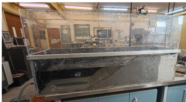
Figure 1: Photograph of reduced scale spoil pile in a box of similar dimensions that the centrifuge box to be used at Southwest Jiaotong University. Pore pressure sensors and laser displacement sensors are installed in the box to refine the installation method and test the response.
