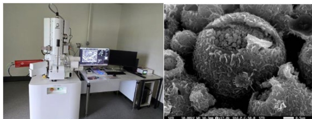
Figure 1: SEM photo of the optimised geopolymers grout
