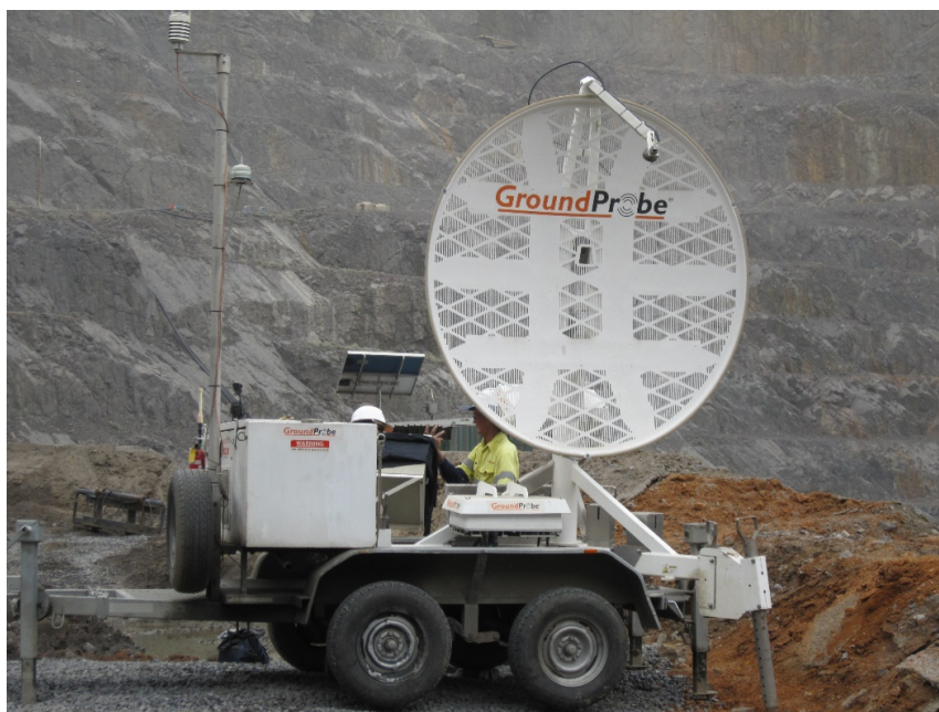
GroundProbe slope stability radar (Photo courtesy of GroundProbe)
