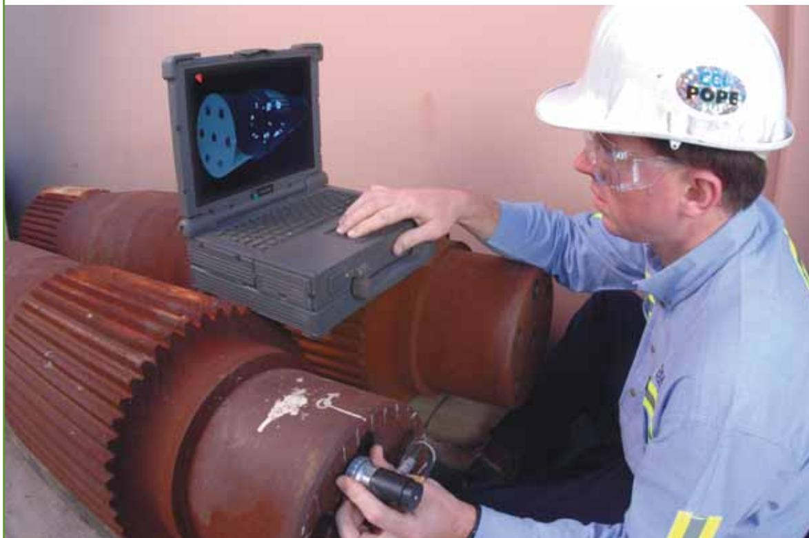
This 3D model – the output of ShafTest™ – confirms the presence of spline cracking defects (multi-coloured patches) in the final drive shafts of a mining shovel.
