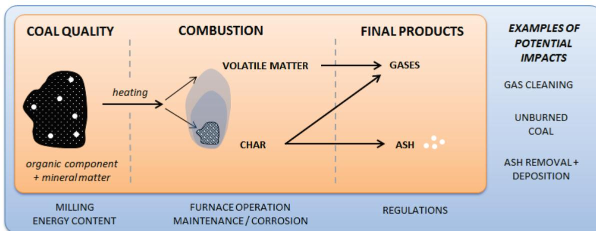
Fig 1: Combustion mechanisms linking coal quality on impacts
